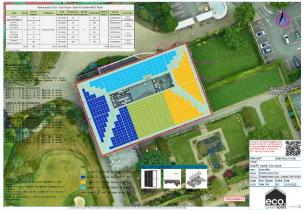
The colours aren't representative of the colour of the panels (they're dark grey) they merely show which panels are connected to which inverters – the electronic devices that take the DC electricity generated by the panels and convert it to 240V AC, just the same as the Grid supply.
